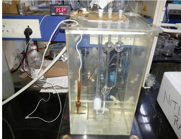
Figure 2. Viscosity measurement of ZnO nanofluid using Borosil Mansingh Survismeter
