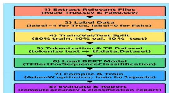
Figure 5: BERT Fine Tuning Pipeline Flow Diagram
